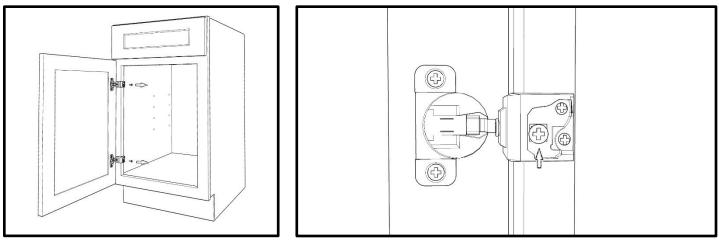
2. Reverse the door panel and drill the 3/4" round head phillips screws to each hinge through the pre-drilled holes to tighten the hinge with cabinet face frame.
