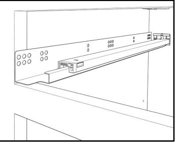
3. Drill two 5/8" flat head Phillips screws at each side to tighten glides and runner profiles to the cabinet face frame.
