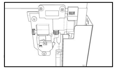
3a. To level the drawer, use the green spur gears on the side to adjust drawer left and right, the green spur gears on the middle to adjust drawer up and down, and the green spur gears on the top to adjust drawer inside and outside.
