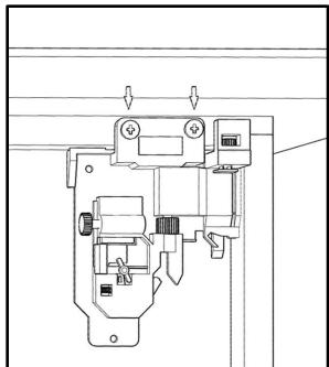
2. Drill two 3/8" flat head phillips screws to each drawer clips to drawer box bottom panel.
