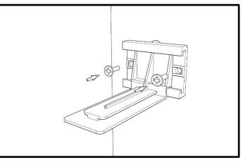
2. Connect glide and runner profiles with each glide base. Slightly pull out the glide to make the other side stay on the middle rail of the cabinet face frame.
