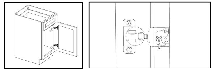
3. If the door is not level when it is installed, the customer will need to turn the screw clockwise to extend the hinge or counterclockwise to shorten the hinge.
